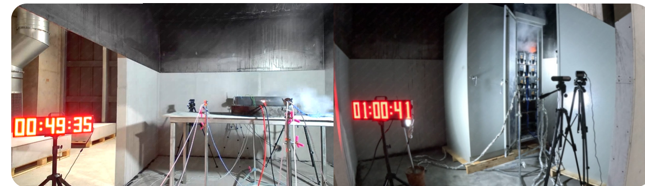
The First Large-Scale Fire Test for a Module-Level Battery and a Unit-Level Lithium Battery Energy Storage System ▲
