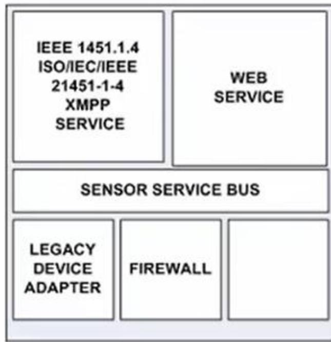
IPDX is the first to offer capabilities based upon the use of XMPP to offer an event driven messaging system for enterprise integration of large scale heterogeneous sensor networks. IPDX offers a distributed decentralized client-server architecture which includes registration, policy administration and management including directory services, data sharing, and security. IPDX provides a reference implementation for the ISO/IEC/IEEE 21451-1-4 standard.
