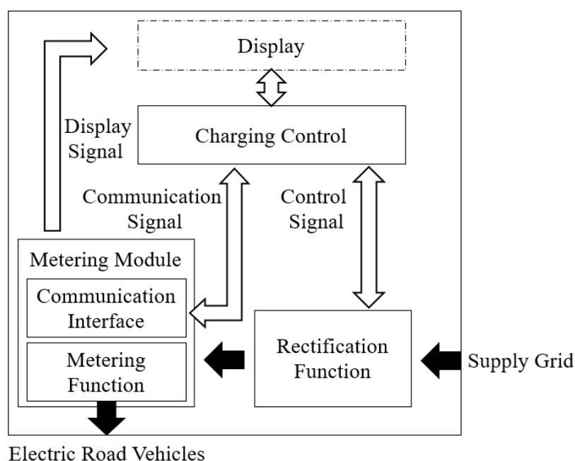
Note: The display can be installed externally or internally in the electric vehicle supply equipment.
