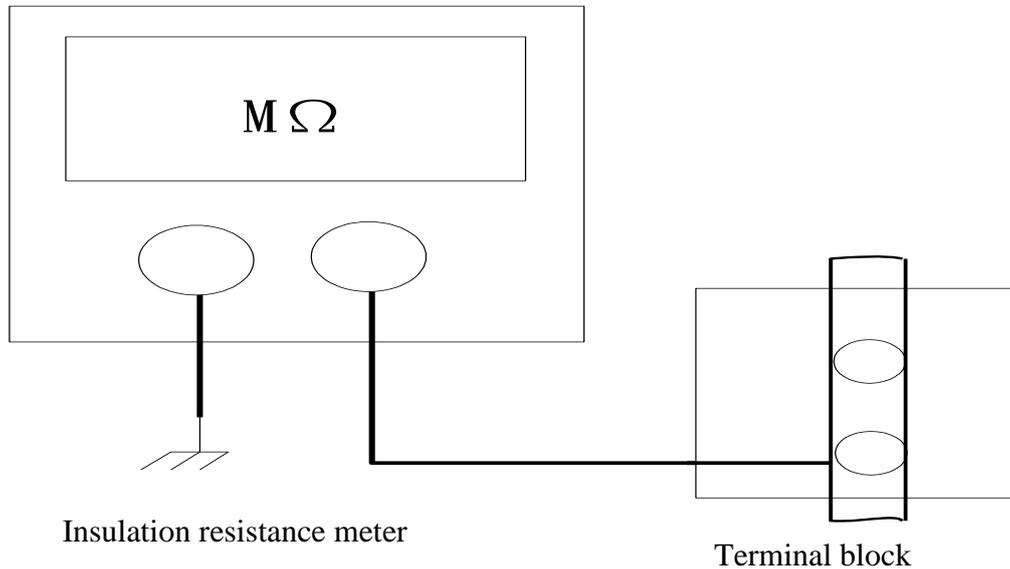
Fig4. Inspection of the insulation resistance value of an inductive loop
