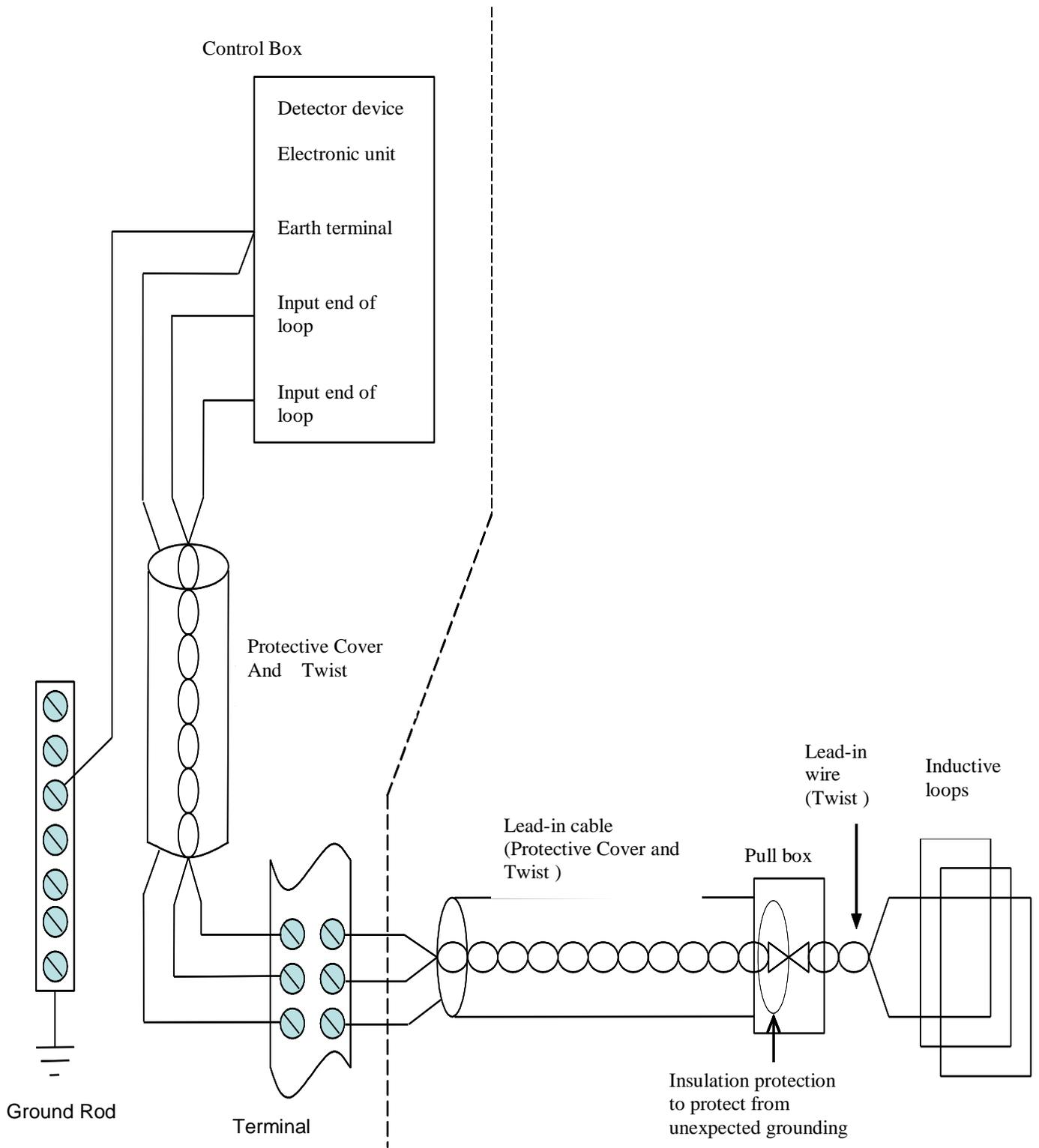
Fig. 1. Installation of inductive loop speedometer
