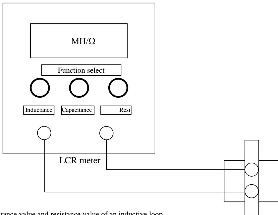
Fig. 3. Inspection of inductance value and resistance value of an inductive loop
