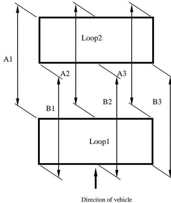
Fig. 2. Distances of A1, A2, A3, B1, B2, and B3, between two sets of inductive loops
