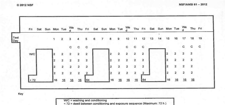
Figure B1 – Exposure sequence for mechanical plumbing device
