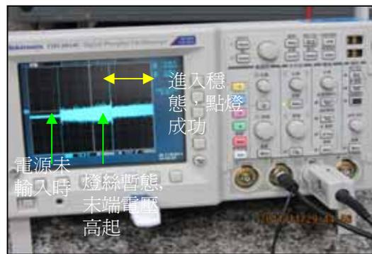
(C)燈管管電壓起動監測(暫態及穩態)
