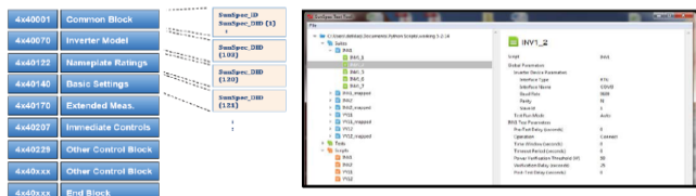
Figure 1: Discrete Inverter Control Blocks
