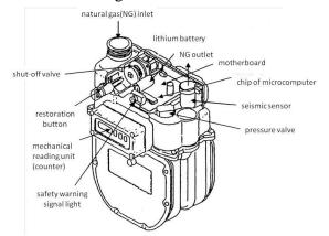
Figure B.1 Structural diagram of a diaphragm gas meter with micro computer
