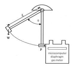
Figure 1 Impact test
