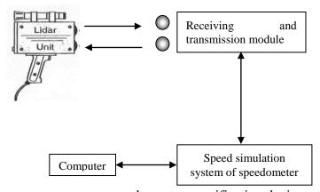
Fig. 4 · speed accuracy verification device
