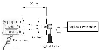
Fig. 3: Optical Power meter verification device
