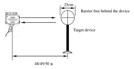
Fig. 1: Rangefinder verification device
