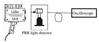
Fig. 2: Laser PRR verification Device
