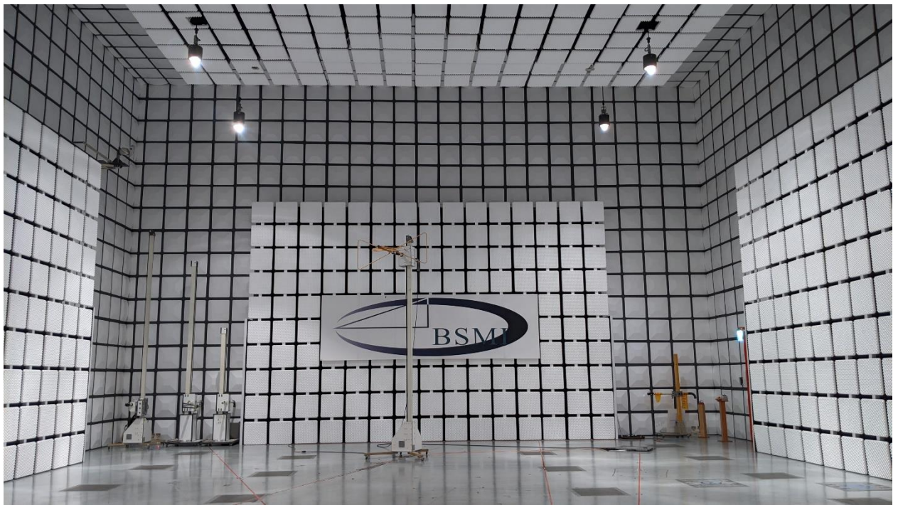
EMC 10m Semi-Anechoic Chamber
