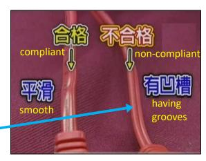
(b) difference between single- and double-layer insulation
