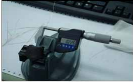
(c)漆包線外徑指的是(導體+膜)厚度
