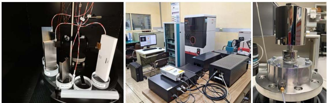
● Gauge Blocks Calibration System - Interferometer
