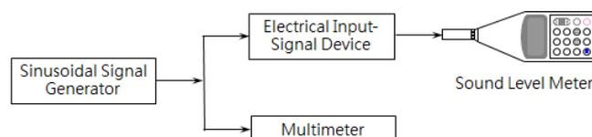
Figure 4 Test system for overload indication of filter
