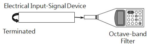
Figure 5 Test system for self-generated noise of filter
