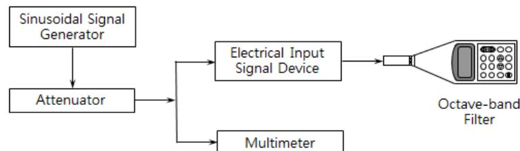
Figure 2 Test system for level linearity of filter
