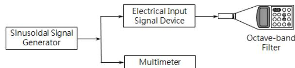
Figure 3 Test system for relative attenuation of filter
