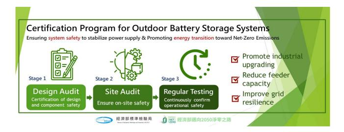
• The Three-Step of Verification Process for Battery Energy Storage System
