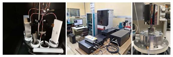
Gauge Blocks Calibration System - Interferometer
