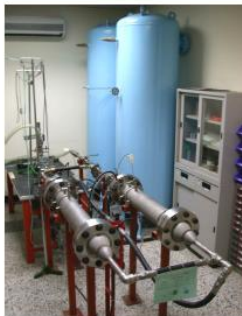
The total volume of the buffer tank is 2.3m 3 .
