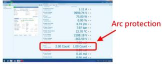
The UXC 1000 will switch off the high voltage and emitter current (water cooling remains on)
