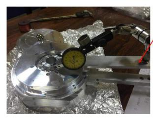
1. Meter mounted on the  $2\theta$  arm 2. Probing the surface of  $\theta$  axis
